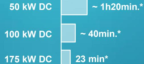
DC Fast charging uses 277/480v, 3 phase power. Breaker amperage is 100A for 50kW and increases to 250A for 175kW
